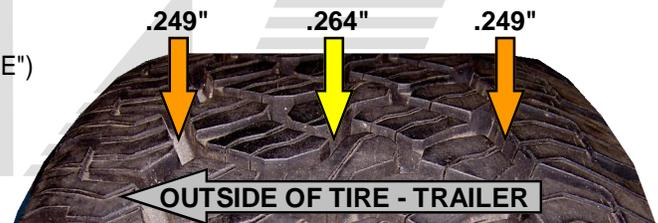
The above shows the center tread *did not* increase wear, but generally the center had *slightly more* tread than the outside edges... most likely due to the shoulders wearing more when turning, so it balances the wear nicely. The front tires indicate they may have had more toe-in than necessary by the outside edge wearing more. Even after a year of continued driving at these elevated pressures and 14,000 miles later, wear across the tread is still exceptionally even.
